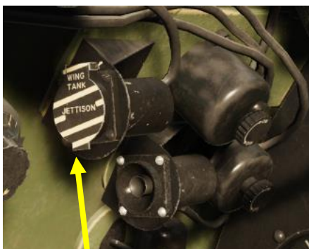
External Wing Fuel Tank Jettison Button Flip safety cover, then press button to jettison external wing fuel tanks
