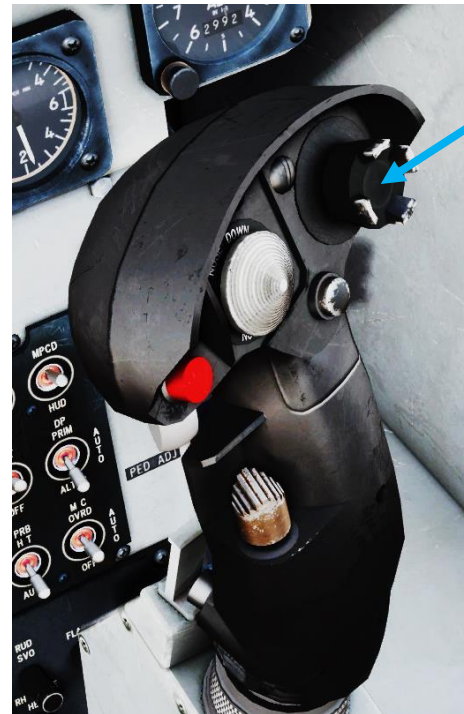
Sensor Select Switch AFT = DMT: LST/TV FWD = INS: IRMV/EOMV LEFT = MAP Center/Decenter RIGHT = FLIR/HUD-BH/WH DOWN (PUSHED) = HUD Scene Reject/TPOD
