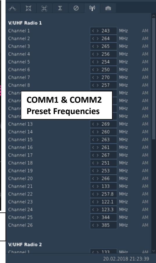
ACNIP (Auxiliary Communication, Navigation, Identification Panel)
