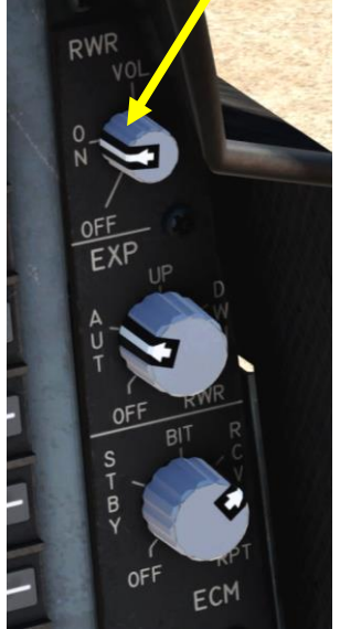
RWR (Radar Warning Receiver) Control Knob OFF / ON / Volume
