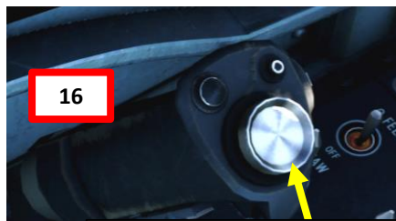
TDC (Target Designation Caret) Control Switch LEFT/RIGHT/FORWARD/AFT/DOWN (ACTION)
